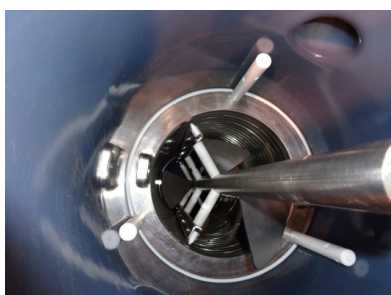
Filter with internal HALAR coating. Basket and cleaning system in Hastelloy.
