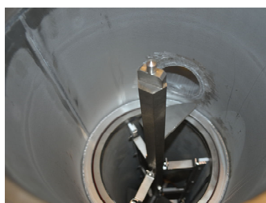
316L-SS filter. Basket and cleaning system in 316L-SS.
